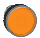
Head for illuminated push button, Harmony XB4, orange flush, 22mm, universal LED, spring return, plain, unmarked
