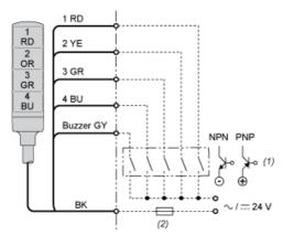
(1) (2) RD : "ON" for lighting and/or applying continuous sound. Fuse (rated current: 0.5 A)
