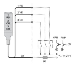
(1) "ON" for lighting and/or applying continuous sound. (2) Fuse (rated current: 0.5 A)
