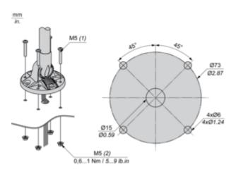
(1) Thickness + 10 mm/0.39 in.(2) Hexagon Nut with flange Ø54 mm/2.13 in., 45°
