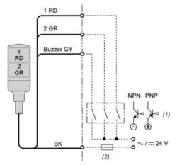
"ON" for lighting and/or applying continuous sound. Fuse (rated current: 0.5 A)
