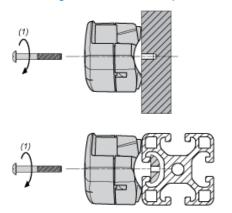
(1) Maximum tightening torque: 0,8 Nm / 7.08 lb-in.
