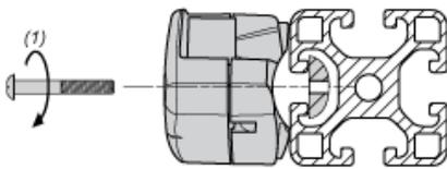
(1) Maximum tightening torque: 0,8 Nm / 7.08 lb-in.
