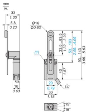
(1) 2 fixing holes  $\text{Ø} 4.2$  mm, counterbored  $\text{Ø} 8$  mm by 4 mm deep.
