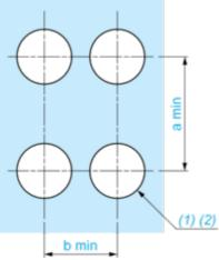
(1) Diameter on finished panel or support (2)  $\emptyset$ 22.5 mm recommended ( $\emptyset$ 22.3  $_0^{+0.4}$ ) /  $\emptyset$ 0.89 in. recommended ( $\emptyset$ 0.88 in.  $_0^{+0.016}$ )
