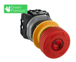
Harmony XB5, Illuminated emergency stop, plastic, red mushroom Ø40, Ø22, trigger latching turn to release, 24 V DC, 1 NO + 2 NC,
