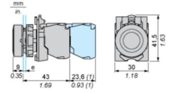
e: clamping thickness: 1 to 6 mm / 0.04 to 0.24 in. (1) Additional row of contacts or double contact
