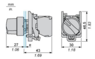
e: clamping thickness: 1 to 6 mm / 0.04 to 0.24 in.
