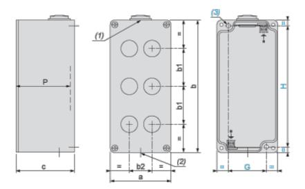
(1): 1 hole, with blanking plug (protrusion 6 mm/0.24 in.), for cable gland ISO M20 x 1.5
