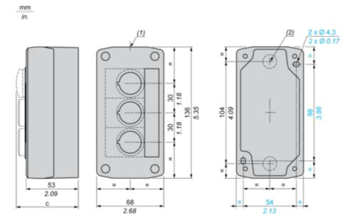
(1) 2 knock-outs for Pg 13.5 cable gland, maximum capacity 12 mm/0.47 in. (2) Knock-out for cable entry, maximum capacity 14 mm/0.55 in.
