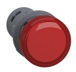
Monolithic pilot light, Easy Harmony XA2, plastic, red, 22mm, integral LED, screw clamp terminals, 380... 400V AC, anti interference
