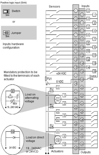
FU1 = 0.5A fast-blow fuse. FU = Fast-blow fuses to be calibrated according to the load. Negative logic input (Source)
