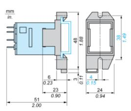
With this mounting type, test button becomes inaccessible.
