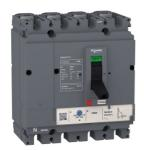
circuit breaker EasyPact CVS250F, 36 kA at 415 VAC, 250 A rating thermal magnetic TM-D trip unit, 4P 3d
