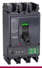
circuit breaker ComPact NSX630N, 50 kA at 415 VAC, MicroLogic 4.3 Vigi trip unit 570 A, 3 poles 3d
