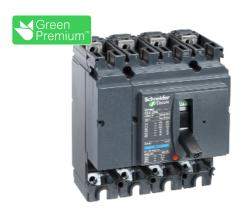
circuit breaker basic frame, Compact NSX250N, 50 kA at 415 VAC 50/60 Hz, 250 A, without trip unit, 4 poles
