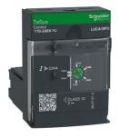
Standard control unit, TeSys U, 4.5-18A, 3P motors, thermal magnetic protection, class 10, coil 110-240V AC/DC
