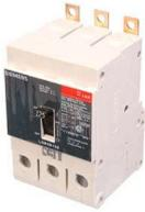
SIEMENS LOW VOLTAGE PANELBOARD MOUNT G FRAME CIRCUIT BREAKER WITH THERMAL - MAGNETIC TRIP UNIT. UL LISTED LGB FRAME WITH VERY HIGH BREAKING CAPACITY. 125A 3-POLE (14KAIC AT 600Y/347V) (65KAIC AT 480Y/277V). SPECIAL FEATURES: LOAD SIDE LUGS ONLY (TC1GG20) WIRE RANGE: 8 - 1/0 AWS (CU/AL). DIMENSIONS (W x H x D) IN: 3 x 5.4 x 2.8.
