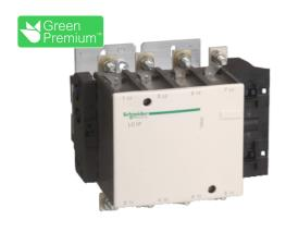
TeSys F contactor - 4P(4 NO)-AC-1 <= 440V 200A with coil LX9 - 24...575V AC 40/400Hz, LX4 -24...460V DC, LXE - 100...250V AC 50/60Hz or 100...380V DC
