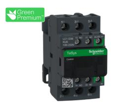
Contactor, TeSys Deca, 3P(3 NO), AC-3/AC-3e, 0 to 440V, 38A, 100 to 250VAC/DC coil
