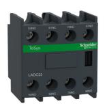
Auxiliary contact block, TeSys D, 2NO + 2NC (inc. 1NO + 1NC make before break), front mounting, screw clamp terminals
