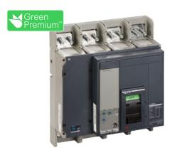
circuit breaker ComPact NS1250N, 50 kA at 415 VAC, Micrologic 2.0 trip unit, 1250 A, fixed,4 poles 4d
