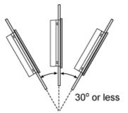
When installing the panel in a slanted position with an incline more than 30°, the ambient temperature must not exceed 40 °C (104 °F). You may need to use forced air cooling (fan,A/C) to ensure the ambient operating temperature is 40°C or less (104 °F or less).
