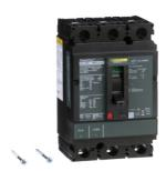
Circuit breaker, PowerPacT H, 70A, 3 pole, 600VAC, 50kA, lugs, thermal magnetic, 80%
