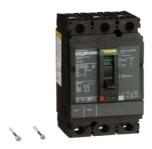
Circuit breaker, PowerPacT H, 20A, 3 pole, 600VAC, 18kA, lugs, thermal magnetic, 80%
