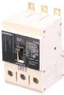
SIEMENS LOW VOLTAGE PANELBOARD MOUNT G FRAME CIRCUIT BREAKER WITH THERMAL - MAGNETIC TRIP UNIT. UL LISTED HGB FRAME WITH HIGH BREAKING CAPACITY. 100A 3-POLE (14KAIC AT 600Y/347V) (35KAIC AT 480Y/277V). SPECIAL FEATURES: LOAD SIDE LUGS ONLY (TC1GG20) WIRE RANGE: 8 - 1/0 AWS (CU/AL). DIMENSIONS (W x H x D) IN: 3 x 5.4 x 2.8.
