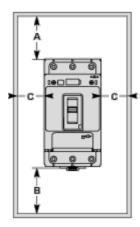
Toggle-type, rotary handle-type: identical clearance values.
