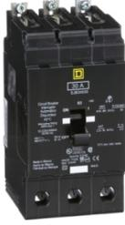
[TAA] Mini circuit breaker, E-Frame, 30A, 3 pole, 480Y/277VAC, 100kA max, bolt on
