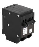
Quad tandem circuit breaker, Homeline Canadian, 2 x 1 pole at 20A, 1 x 2 pole at 30A, 120/240VAC, 10kA AIR, plug in, UL
