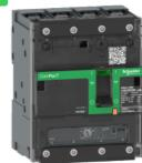
Circuit breaker, ComPacT NSXm 160F, 36kA/415VAC, 4 poles 3D (neutral not protected), TMD trip unit 125A, lugs/busbars
