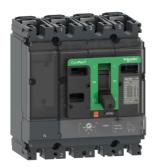
Circuit breaker, ComPacT NSX100H, 70kA/415VAC, 4 poles 3D (neutral not protected), TMD trip unit 40A
