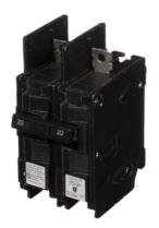
Siemens Low Voltage Molded Case Circuit Breakers General Purpose MCCBs - Type BQ, 2-Pole, 120/240VAC are Circuit Protection Molded Case Circuit Breakers. 2-Pole Common-Trip circuit breaker type BQH. Rated 120/240V (020A) (AIR 22 kA). Special features: Load side lugs are included.
