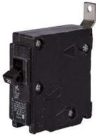
Siemens Low Voltage Molded Case Circuit Breakers Panelboard Mounting 240V Circuit Breakers - Type BL, 1-Pole, 120VAC are Circuit Protection Molded Case Circuit Breakers. Type: HBL Application: Electrical Distribution Standard: UL 489 Voltage Rating: 120V Amperage Rating: 15A Trip Range: Thermal Magnetic Interrupt Rating: 65 AIC Number Of Poles: 1P
