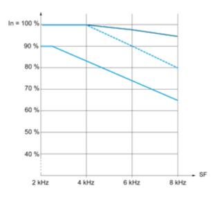
40 °C (104 °F) - Mounting type A, B and C 50 °C (122 °F) - Mounting type A, B and C 60 °C (140 °F) - Mounting type B and C In : Nominal Drive Current
