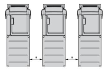
Frame sizes 1, 2, 3, 3S and 5S:  $a \ge 100 \text{ mm} (3.9 \text{ in.})$ Frame sizes 4, 5 and 6:  $a \ge 110 \text{ mm} (4.33 \text{ in.})$
