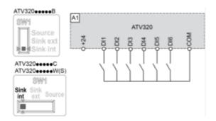
Switch SW1 set to "Sink Ext" position and use of an external power supply for the Dls.
