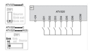
Switch SW1 set to "Sink Ext" position and use of an external power supply for the Dls.
