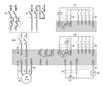
Drive Contactor (only if a control circuit is needed) 2.2 k $\Omega$  reference potentiometer. This can be replaced by a 10 k $\Omega$  potentiometer (maximum). Circuit breaker Negative logic (Sink) Positive logic (Source) (factory set configuration) 0...10 V or 0...20 mA
