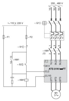
(1) A1 : A line contactor must be used in the sequence.
