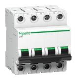
Miniature circuit breaker (MCB), Acti9 xC60, 4P, 6A, C curve, 10000A (IS/IEC60898-1)
