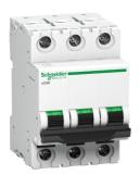
Miniature circuit breaker (MCB), Acti9 xC60, 3P, 6A, C curve, 10000A (IS/IEC60898-1)
