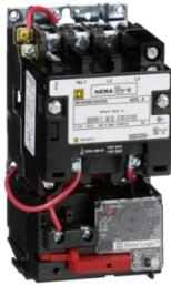
NEMA motor starter, Type S, nonreversing, Size 0, 18A, 5HP at 460VAC, up to 100kA SCCR, 3 phase, 3 pole, Motor Logic, 120VAC coil, open
