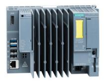
SIMATIC ET 200SP Open Controller, CPU 1515SP PC2 F, 8 GB RAM (basic device 6ES7677-2DB40-0AA0), 128 GB CFast with Windows 10 IoT Enterprise LTSC 2019 64-bit and S7-1500 Failsafe Software Controller CPU 1505SP F V2x preinstalled; interfaces: 1x slot CFast, 1x slot SD/MMC, 1x connection for ET 200SP BusAdapter PROFINET, 1x 10/100/1000 Mbps Ethernet, 2x USB 3.0, 2x USB 2.0, 1x DisplayPort; documentation on CFast, restore image on CFast
