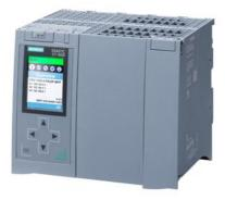
SIMATIC S7-1500, CPU Bundle consisting of: CPU 1518-4 PN/DP MFP (6ES7518-4AX00-1AB0), including C/C++ Runtime and OPC UA Runtime license, 6 MB work memory for program and 60 MB for data, 1st interface: PROFINET IRT with 2-port switch, 2nd interface: PROFINET RT, 3rd interface: PROFINET basic services, 4th interface: PROFIBUS, 1 ns bit performance, SIMATIC Memory Card (min. 2 GB) required
