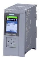
SIMATIC S7-1500F, CPU 1516F-3 PN/DP, central processing unit with work memory 3 MB for program and 7.5 MB for data 1st interface: PROFINET IRT with 2-port switch, 2nd interface: PROFINET RT, 3rd interface: PROFIBUS, 6 ns bit performance, SIMATIC Memory Card required \*\*\*\*approvals and certificates according to entry 109817466 at support.industry.siemens.com to be considered! -
