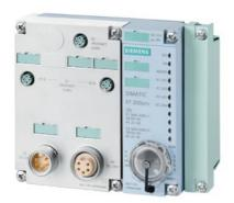
SIMATIC DP, CPU 1516PRO-2 PN for ET 200pro, Central processing unit with Work memory 1 MB for program and 5 MB for data, 1st interface: PROFINET IRT with 3-port switch, 2nd interface: PROFINET RT, 10 ns bit performance, degree of protection: IP65/67, SIMATIC Memory Card required, Connection module required
