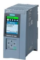
SIMATIC S7-1500R, CPU 1515R-2 PN central processing unit with work memory 1 MB for program and 4.5 MB for data, 1st interface: PROFINET RT with 2-port switch, 2nd interface: PROFINET, SIMATIC Memory Card required
